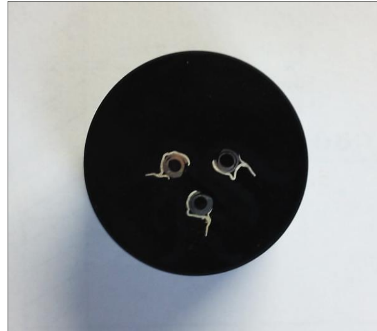
Example of improperly installed Spring Energized Seal (Jacket stripped from spring)
