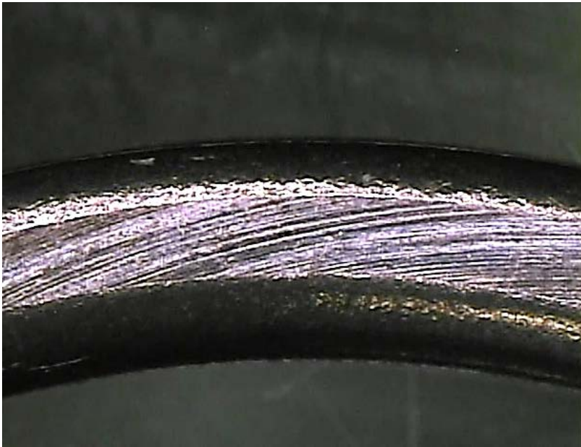
Silver Plating: O-Ring Poor Flange Finish: Radial Marks
