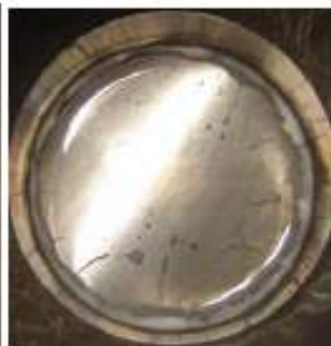
Typical leakage through poorly sealed coating
