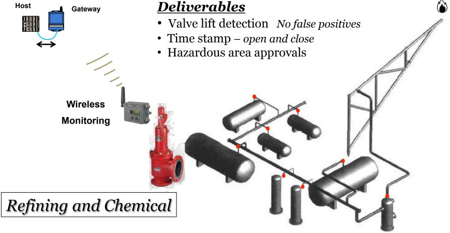
Schematic of a relief valve system showing pressure vessels, relief valves, relief header, vent scrubber and vent boom. Process piping has been omitted for clarity.
