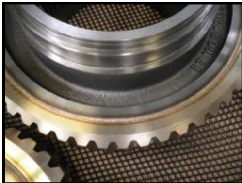
Bronze welded worm wheel (source: AUMA)
