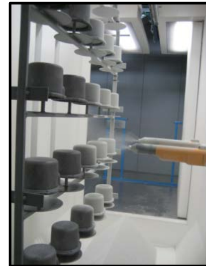
Powder coating process (source: AUMA)
