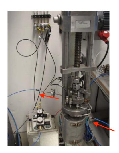
Inlet flushing gas
