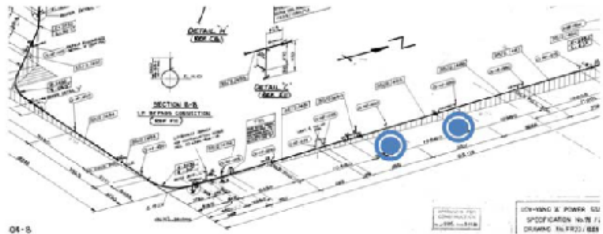
Figure 4. Summary of problem areas on Unit 2 HRH horizontal line 4
