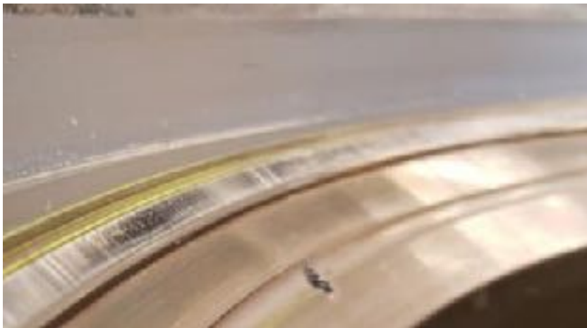
K-EI 850® coated seat after endurance test
