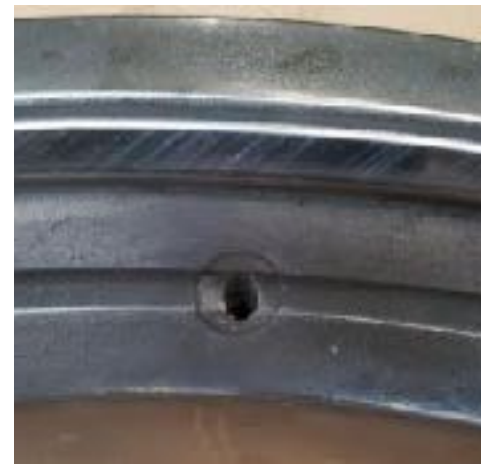
Tungsten Carbide coated seat after endurance test
