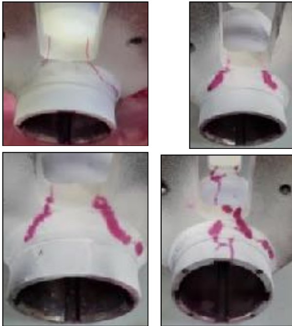
Crack position highlighted by PT test.
