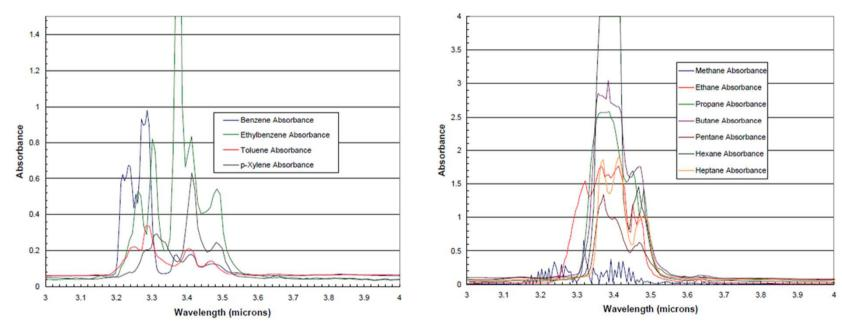
Figure 1. Aromatic Compound IR Absorbance.
