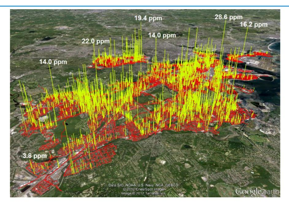
Over 3000 methane leaks were discovered (yellow) over Boston's 785 mile road network (red) in a 2012
